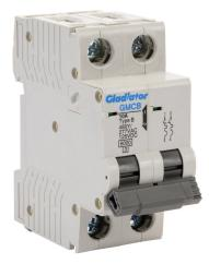
Gladiator miniature supplementary protector, 10A, 480Y / 277 VAC / 125 VDC, 2-pole, B curve, thermal magnetic, 6kA @ 480Y/277 VAC interrupting rating, 35mm DIN rail mount.
