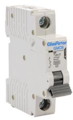
Gladiator miniature supplementary protector, 8A, 277 VAC / 60 VDC, 1-pole, D curve, thermal magnetic, 6kA @ 277 VAC interrupting rating, 35mm DIN rail mount.
