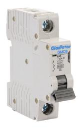
Gladiator miniature supplementary protector, 63A, 277 VAC / 60 VDC, 1-pole, D curve, thermal magnetic, 6kA @ 277 VAC interrupting rating, 35mm DIN rail mount.
