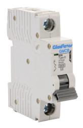
Gladiator miniature supplementary protector, 50A, 277 VAC / 60 VDC, 1-pole, D curve, thermal magnetic, 6kA @ 277 VAC interrupting rating, 35mm DIN rail mount.
