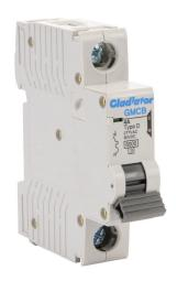
Gladiator miniature supplementary protector, 4A, 277 VAC / 60 VDC, 1-pole, D curve, thermal magnetic, 6kA @ 277 VAC interrupting rating, 35mm DIN rail mount.
