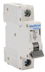
Gladiator miniature supplementary protector, 40A, 277 VAC / 60 VDC, 1-pole, D curve, thermal magnetic, 6kA @ 277 VAC interrupting rating, 35mm DIN rail mount.
