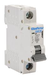
Gladiator miniature supplementary protector, 3A, 277 VAC / 60 VDC, 1-pole, D curve, thermal magnetic, 6kA @ 277 VAC interrupting rating, 35mm DIN rail mount.
