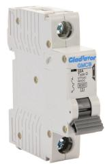
Gladiator miniature supplementary protector, 32A, 277 VAC / 60 VDC, 1-pole, D curve, thermal magnetic, 6kA @ 277 VAC interrupting rating, 35mm DIN rail mount.
