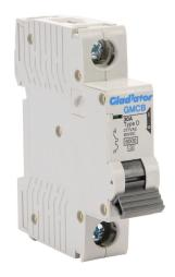
Gladiator miniature supplementary protector, 30A, 277 VAC / 60 VDC, 1-pole, D curve, thermal magnetic, 6kA @ 277 VAC interrupting rating, 35mm DIN rail mount.
