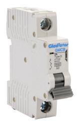
Gladiator miniature supplementary protector, 2A, 277 VAC / 60 VDC, 1-pole, D curve, thermal magnetic, 6kA @ 277 VAC interrupting rating, 35mm DIN rail mount.
