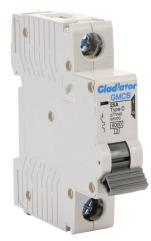
Gladiator miniature supplementary protector, 25A, 277 VAC / 60 VDC, 1-pole, D curve, thermal magnetic, 6kA @ 277 VAC interrupting rating, 35mm DIN rail mount.
