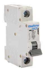
Gladiator miniature supplementary protector, 20A, 277 VAC / 60 VDC, 1-pole, D curve, thermal magnetic, 6kA @ 277 VAC interrupting rating, 35mm DIN rail mount.
