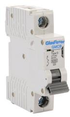
Gladiator miniature supplementary protector, 1A, 277 VAC / 60 VDC, 1-pole, D curve, thermal magnetic, 6kA @ 277 VAC interrupting rating, 35mm DIN rail mount.
