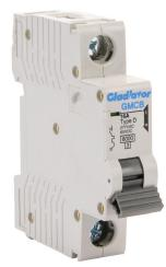
Gladiator miniature supplementary protector, 16A, 277 VAC / 60 VDC, 1-pole, D curve, thermal magnetic, 6kA @ 277 VAC interrupting rating, 35mm DIN rail mount.
