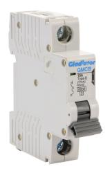
Gladiator miniature supplementary protector, 15A, 277 VAC / 60 VDC, 1-pole, D curve, thermal magnetic, 6kA @ 277 VAC interrupting rating, 35mm DIN rail mount.
