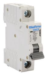
Gladiator miniature supplementary protector, 10A, 277 VAC / 60 VDC, 1-pole, D curve, thermal magnetic, 6kA @ 277 VAC interrupting rating, 35mm DIN rail mount.
