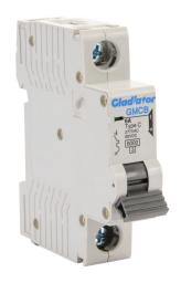
Gladiator miniature supplementary protector, 6A, 277 VAC / 60 VDC, 1-pole, C curve, thermal magnetic, 6kA @ 277 VAC interrupting rating, 35mm DIN rail mount.
