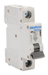
Gladiator miniature supplementary protector, 63A, 277 VAC / 60 VDC, 1-pole, C curve, thermal magnetic, 6kA @ 277 VAC interrupting rating, 35mm DIN rail mount.
