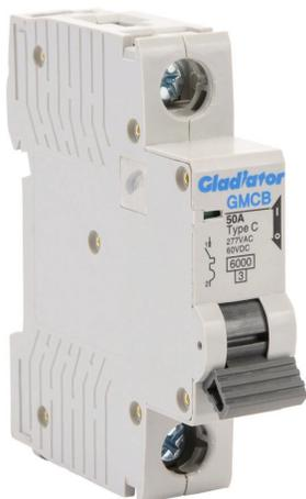
Gladiator miniature supplementary protector, 50A, 277 VAC / 60 VDC, 1-pole, C curve, thermal magnetic, 6kA @ 277 VAC interrupting rating, 35mm DIN rail mount.
