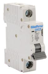
Gladiator miniature supplementary protector, 4A, 277 VAC / 60 VDC, 1-pole, C curve, thermal magnetic, 6kA @ 277 VAC interrupting rating, 35mm DIN rail mount.
