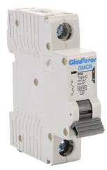
Gladiator miniature supplementary protector, 40A, 277 VAC / 60 VDC, 1-pole, C curve, thermal magnetic, 6kA @ 277 VAC interrupting rating, 35mm DIN rail mount.
