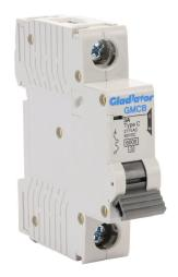
Gladiator miniature supplementary protector, 3A, 277 VAC / 60 VDC, 1-pole, C curve, thermal magnetic, 6kA @ 277 VAC interrupting rating, 35mm DIN rail mount.
