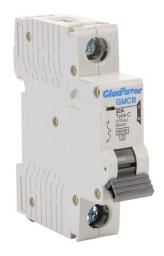
Gladiator miniature supplementary protector, 32A, 277 VAC / 60 VDC, 1-pole, C curve, thermal magnetic, 6kA @ 277 VAC interrupting rating, 35mm DIN rail mount.
