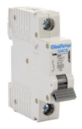
Gladiator miniature supplementary protector, 30A, 277 VAC / 60 VDC, 1-pole, C curve, thermal magnetic, 6kA @ 277 VAC interrupting rating, 35mm DIN rail mount.
