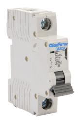
Gladiator miniature supplementary protector, 2A, 277 VAC / 60 VDC, 1-pole, C curve, thermal magnetic, 6kA @ 277 VAC interrupting rating, 35mm DIN rail mount.
