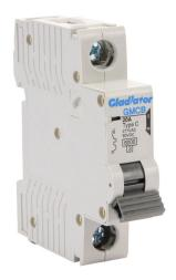
Gladiator miniature supplementary protector, 20A, 277 VAC / 60 VDC, 1-pole, C curve, thermal magnetic, 6kA @ 277 VAC interrupting rating, 35mm DIN rail mount.
