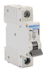
Gladiator miniature supplementary protector, 1A, 277 VAC / 60 VDC, 1-pole, C curve, thermal magnetic, 6kA @ 277 VAC interrupting rating, 35mm DIN rail mount.
