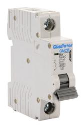
Gladiator miniature supplementary protector, 16A, 277 VAC / 60 VDC, 1-pole, C curve, thermal magnetic, 6kA @ 277 VAC interrupting rating, 35mm DIN rail mount.
