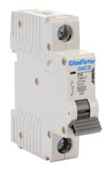
Gladiator miniature supplementary protector, 15A, 277 VAC / 60 VDC, 1-pole, C curve, thermal magnetic, 6kA @ 277 VAC interrupting rating, 35mm DIN rail mount.
