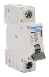
Gladiator miniature supplementary protector, 10A, 277 VAC / 60 VDC, 1-pole, C curve, thermal magnetic, 6kA @ 277 VAC interrupting rating, 35mm DIN rail mount.
