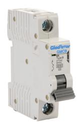
Gladiator miniature supplementary protector, 8A, 277 VAC / 60 VDC, 1-pole, B curve, thermal magnetic, 6kA @ 277 VAC interrupting rating, 35mm DIN rail mount.
