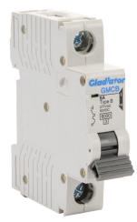
Gladiator miniature supplementary protector, 6A, 277 VAC / 60 VDC, 1-pole, B curve, thermal magnetic, 6kA @ 277 VAC interrupting rating, 35mm DIN rail mount.
