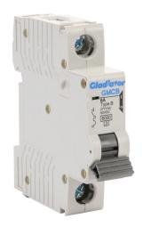
Gladiator miniature supplementary protector, 6A, 277 VAC / 60 VDC, 1-pole, B curve, thermal magnetic, 6kA @ 277 VAC interrupting rating, 35mm DIN rail mount.
