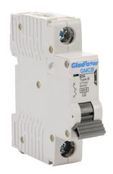
Gladiator miniature supplementary protector, 63A, 277 VAC / 60 VDC, 1-pole, B curve, thermal magnetic, 6kA @ 277 VAC interrupting rating, 35mm DIN rail mount.
