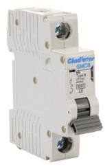
Gladiator miniature supplementary protector, 5A, 277 VAC / 60 VDC, 1-pole, B curve, thermal magnetic, 6kA @ 277 VAC interrupting rating, 35mm DIN rail mount.
