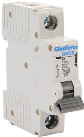
Gladiator miniature supplementary protector, 4A, 277 VAC / 60 VDC, 1-pole, B curve, thermal magnetic, 6kA @ 277 VAC interrupting rating, 35mm DIN rail mount.
