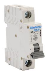
Gladiator miniature supplementary protector, 4A, 277 VAC / 60 VDC, 1-pole, B curve, thermal magnetic, 6kA @ 277 VAC interrupting rating, 35mm DIN rail mount.
