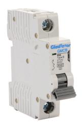
Gladiator miniature supplementary protector, 40A, 277 VAC / 60 VDC, 1-pole, B curve, thermal magnetic, 6kA @ 277 VAC interrupting rating, 35mm DIN rail mount.
