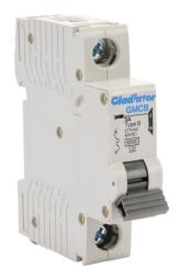
Gladiator miniature supplementary protector, 3A, 277 VAC / 60 VDC, 1-pole, B curve, thermal magnetic, 6kA @ 277 VAC interrupting rating, 35mm DIN rail mount.
