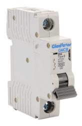
Gladiator miniature supplementary protector, 32A, 277 VAC / 60 VDC, 1-pole, B curve, thermal magnetic, 6kA @ 277 VAC interrupting rating, 35mm DIN rail mount.
