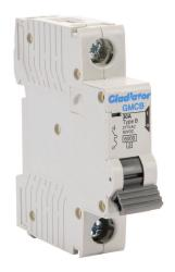
Gladiator miniature supplementary protector, 30A, 277 VAC / 60 VDC, 1-pole, B curve, thermal magnetic, 6kA @ 277 VAC interrupting rating, 35mm DIN rail mount.
