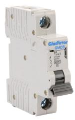
Gladiator miniature supplementary protector, 2A, 277 VAC / 60 VDC, 1-pole, B curve, thermal magnetic, 6kA @ 277 VAC interrupting rating, 35mm DIN rail mount.
