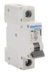
Gladiator miniature supplementary protector, 25A, 277 VAC / 60 VDC, 1-pole, B curve, thermal magnetic, 6kA @ 277 VAC interrupting rating, 35mm DIN rail mount.
