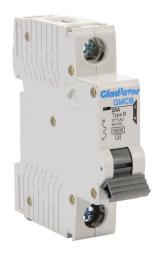
Gladiator miniature supplementary protector, 20A, 277 VAC / 60 VDC, 1-pole, B curve, thermal magnetic, 6kA @ 277 VAC interrupting rating, 35mm DIN rail mount.
