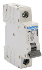
Gladiator miniature supplementary protector, 1A, 277 VAC / 60 VDC, 1-pole, B curve, thermal magnetic, 6kA @ 277 VAC interrupting rating, 35mm DIN rail mount.
