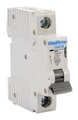
Gladiator miniature supplementary protector, 16A, 277 VAC / 60 VDC, 1-pole, B curve, thermal magnetic, 6kA @ 277 VAC interrupting rating, 35mm DIN rail mount.
