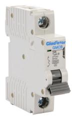
Gladiator miniature supplementary protector, 15A, 277 VAC / 60 VDC, 1-pole, B curve, thermal magnetic, 6kA @ 277 VAC interrupting rating, 35mm DIN rail mount.
