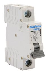
Gladiator miniature supplementary protector, 10A, 277 VAC / 60 VDC, 1-pole, B curve, thermal magnetic, 6kA @ 277 VAC interrupting rating, 35mm DIN rail mount.
