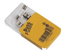
Bussmann fuse, GMC series, small dimension, medium time-delay, 4A, 125 VAC, glass tube. Package of 5. Supplemental, electronic protection applications. Manufacturer part number: GMC-4A-R.
