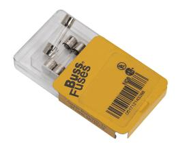
Bussmann fuse, GMC series, small dimension, medium time-delay, 3A, 250 VAC, glass tube. Package of 5. Supplemental, electronic protection applications. Manufacturer part number: GMC-3A-R.
