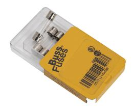
Bussmann fuse, GMC series, small dimension, medium time-delay, 10A, 125 VAC, glass tube. Package of 5. Supplemental, electronic protection applications. Manufacturer part number: GMC-10A-R.
