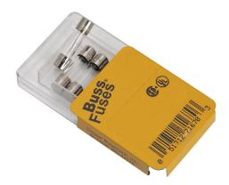
Bussmann fuse, GMA series, small dimension, fast-acting, 5A, 125 VAC, glass tube. Package of 5. Supplemental, electronic protection applications. Manufacturer part number: GMA-5A-R.
